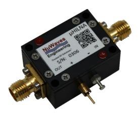
Figure 1. NuWaves' µHILNA<sup>™</sup> Low Noise Amplifier (LNA) operates from 50 to 1500 MHz, delivers 20 dB of gain, with less than 1 dB of Noise Figure (NF) and a Third-Order Intermodulation Product (IP3) of +31 dBm.
