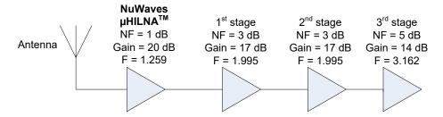
Figure 3. The μHILNA<sup>™</sup> is inserted between the antenna and the notional receiver, improving the NF of the system by approximately 2 dB.
