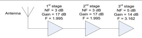
Figure 2. The notional receiver used as an example in this application note has a first stage NF of 3 dB.
