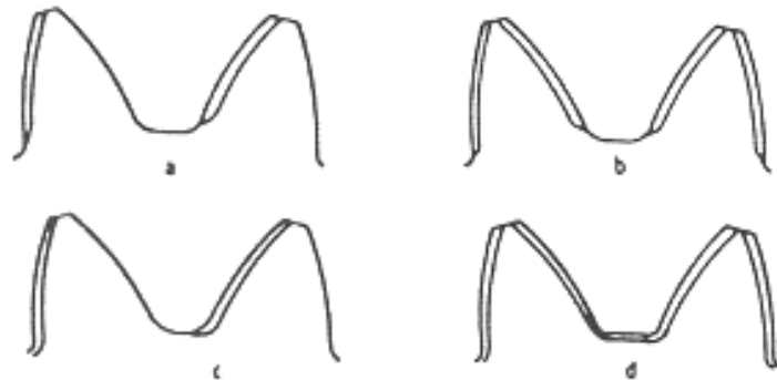
Fig. 4.37 Different Chamfer Forms by Rotary Chamfering and Deburring
