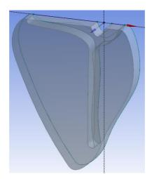
Add a third sketch in the XY Plane. Draw a **circle** that completely surrounds the steak. This circle will form the surface of the pan where the heat will be applied. Extrude this circle by selecting **Add Frozen** in the **Reverse Direction** by 0.5 cm. and click **Generate**.
