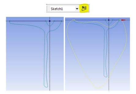
Now draw the meat part by using the **Spline** tool. To end the spline, right-click and select **Closed End**. Do not make the meat go beyond the bone at the top. See figure above (right). This will ensure a clean Boolean subtraction in the next step.
