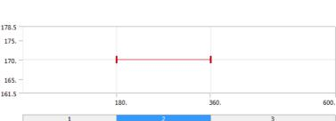
other frying pan body. You will also need to set it so that the temperature is only applied during the second step (180-360 seconds).
