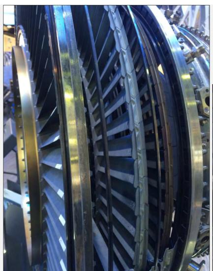
Titanium Aluminide can replace Nickel based materials in the final stages of the low pressure turbine (LPT)
