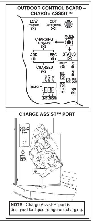
*NOTE:* Outdoor Temperature (ODT) must be between 55°F and 120°F. See Section 14.1
