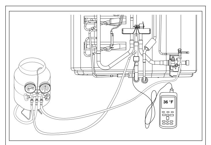
**STEP 3** - Measure the suction line pressure and temperature at the "true" suction line and record the values below.
