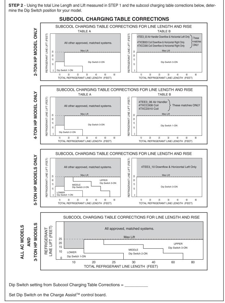
Final refrigerant charge adjustment is necessary. Choose the appropriate method below.
