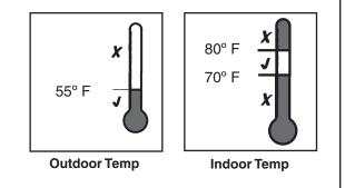
**STEP 2** - Stabilize the system by operating in the heating mode for a minimum of 20 minutes.
