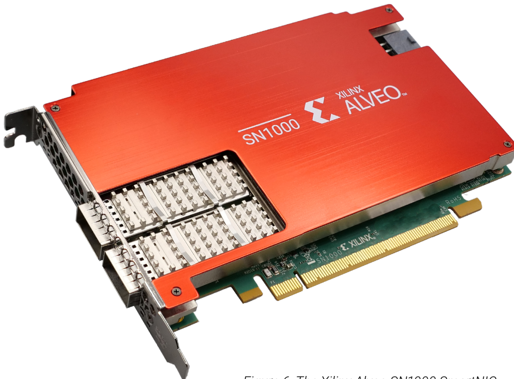
Figure 6: The Xilinx Alveo SN1000 SmartNIC
