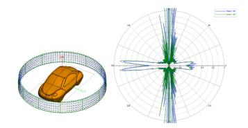
Figure 4: Feko-calculated RCS information can be included in a WinProp simulation through .ffe file import.
