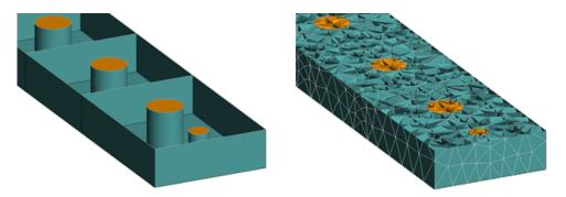
Figure 20: Partial view of a coaxial diplexer model (left) and mesh (right) with the perfect electric conductor pins meshed into tetrahedra with the dielectrics and solved as part of the FEM solution.
