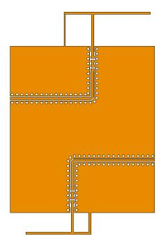
Figure 12: View of an exported Gerber file of a planar antenna with via holes.
