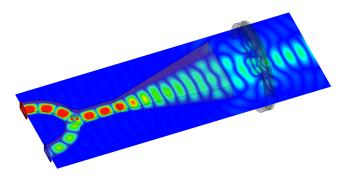
Figure 15: Ferrite circulator (FEM) with horn antenna and dielectric lens (SEP).
