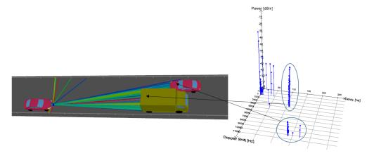
Figure 9: An automotive radar simulation in Altair WinProp.
