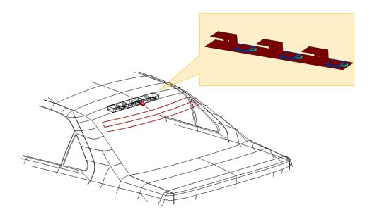
Figure 11: Partial view of a car with a windscreen antenna solved with the MoM/MLFMM and an antenna module mounted in the car's roof (shown enlarged in the insert) solved with the FEM.
