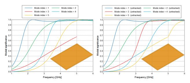
Figure 19: Modal significance plots from a characteristic mode analysis performed on a PEC plate showing tracked modes on the left and untracked results on the right.
