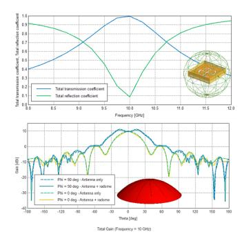
Figure 14: Antenna operating at 10 GHz with FSS radome modelled with a characterised surface. The radome simulation completes within a few minutes.
