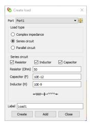
Figure 7: The Create load dialog now shows an image of the resulting circuit.
