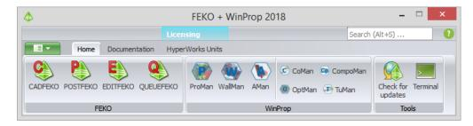
Figure 13: The Feko + WinProp Launcher utility
