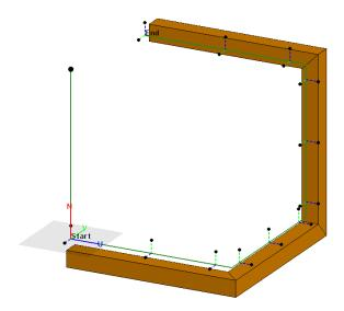
Figure 16: A reference direction can be defined to specify the orientation of a cable.
