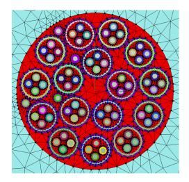
Figure 17: An example of a cable cross section mesh used by the solver.
