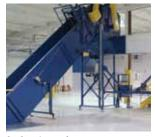
**Conveyors** Allegheny offers Sorting Conveyors, which allow several operators to separate materials by grade and type prior to shredding to maximize the value of your recycled paper. We also offer Primary Conveyors (in-floor or above-ground), Metering Conveyors (seeAuto-Feed<sup>TM</sup> Systems
