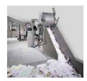
**Auto-Feed™ Systems** Allegheny's revolutionary Auto-Feed<sup>TM</sup> Systems greatly increase your shredding capacity while significantly reducing your labor costs. These systems utilize a high capacity Primary Conveyor (in-floor or above-ground) coupled with a variable-speed Metering Conveyor,
