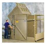
**Tippers** Used with a loading cart, security container, or a Gaylord box, Allegheny Tippers offer an efficient way to load material onto your shredder's input conveyor. This increases the volume of throughput to be shredded and minimizes operator fatigue and strain.
