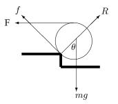
Let the angle between the radius to the point of contact with the step and the downward vertical be  $\theta$ , as shown. At the point of contact, let the frictional force, which is tangent to the sphere, be *f* and the reaction *R* (along the radius of the sphere).
