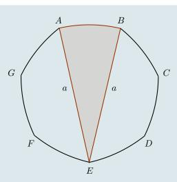
The diagram shows a British 50 pence coin. The seven arcs AB, BC, ..., FG, GA are of equal length and each arc is formed from the circle of radius a having its centre at the vertex diametrically opposite the mid-point of the arc. Show that the area of the face of the coin is
