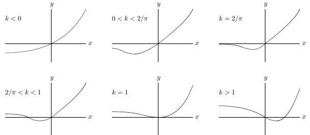
As you see, the equation  $(e^x - 1) - k \tan^{-1} x = 0$  has one root if  $k \leq \frac{1}{2}\pi$  and two roots otherwise. The case k = 1 can be thought of as having one root at x = 0 or as having two roots, both at x = 0 (it is a double root).
