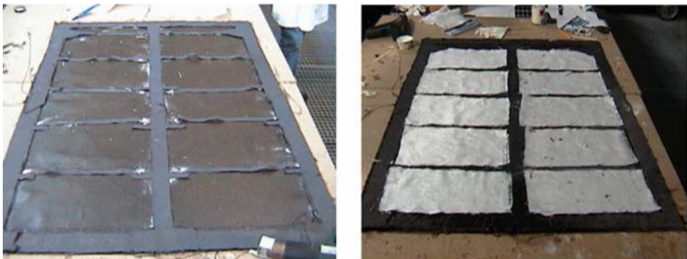
Figure 13. Particular of preform preparation. On the right: glass layers used to replace the syntactic foam of the original component.
