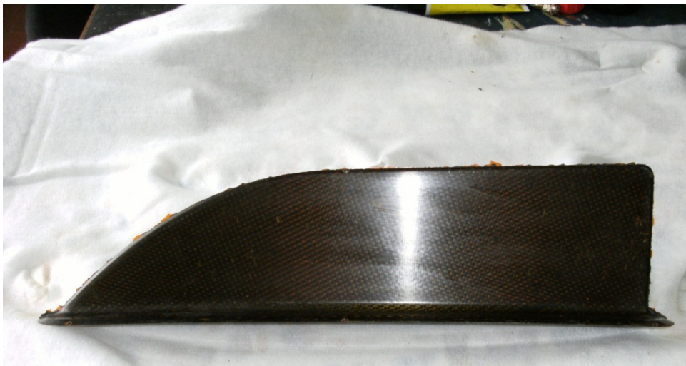
Figure 9. Strake of Aermacchi nacelles after demolding.
