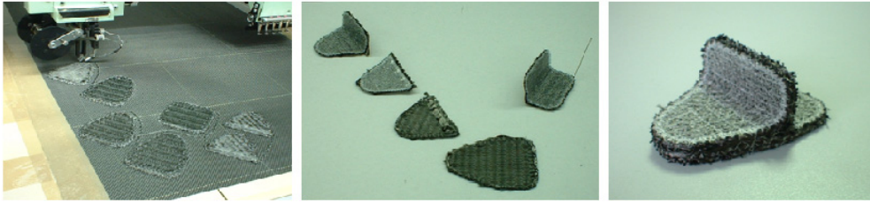
Figure 15. Realization of the preform: cut and stitching.
