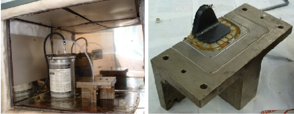
Figure 16. Realization of the bracket by RTM process: resin injection (left), bracket demolded (right).
