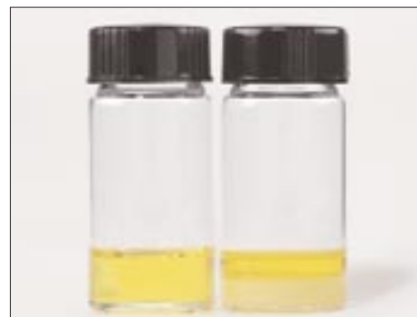
Figure 3. (l) Nanofiller in Adper™ Scotchbond™ 1 XT Adhesive remains in solution; (r) filler in Optibond Solo Plus™ does not.
