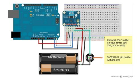
Be careful inserting noisy loads that can cause a sharp current draw, such as DC motors, since they can cause problems on the power lines and may cause the INA219 to reset, etc. When using a DC motor or a similar device, be sure to include a large capacitor to decouple the motor from the power supply and use a snubber diode to protect against inductive spikes.
