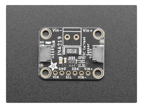
The INA219B breakout board and the INA219 FeatherWing will solve all your power-monitoring problems. Instead of struggling with two multimeters, you can use this breakout to measure both the high side voltage and DC current draw over I2C with 1% precision.
