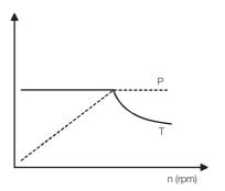
Figure 6.4 Typical torque and power curves in a constant power/torque application.
