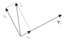
Figure 4.4 Stator current ( $i_{s}$ ) consists of reactive current ( $i_{sd}$ ) and active current ( $i_{sq}$ ) components which are perpendicular to each other. Stator flux is denoted as  $\psi_{s}$ .
