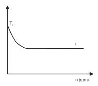
Figure 6.5 Typical torque curve in an application where starting torque is needed.
