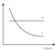
Figure 6.3 Typical torque and power curves in a constant power application.
