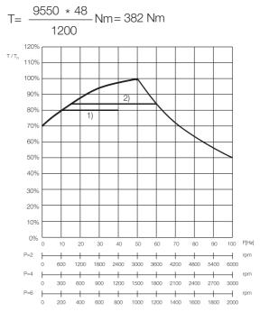
Figure 8.2 Motor loadability curves in a constant torque application. comparison of 1) 4-pole and 2) 6-pole motors.
