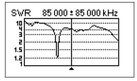
You may set the center frequency (the 2 key) or scanning range (the 3 key). By using arrow keys, these parameters may be increased or decreased.
