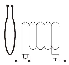
A one-turn coil (about 10 cm in diameter) connected to the analyzer was placed, coaxially, a few centimeters away from the measured trap. The SWR graph shows a visible dip near 17.8 MHz, which is a resonant frequency of the trap.
