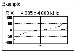
The 1/4-wave resonant frequency of the piece of open-circuited RG-58 cable is 4835 kHz
