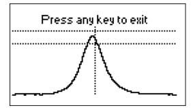
The top of the curve should be located in the middle of the screen, between the two horizontal dotted lines. A small horizontal shift of the curve is allowed.
