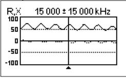
3. Changing the display range and performing additional scans, find a frequency where R (solid line) reaches its maximum, and another frequency with minimum. At these points, X (dotted line) will cross the zero line.
