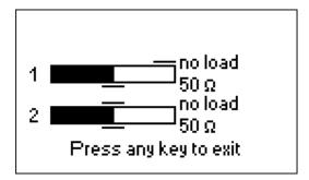
If the bars are not filled at all, the RF output stage or/and the detector are not working properly in the analyzer.
