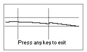
The voltage curve should stay between the horizontal dotted lines. The vertical lines are the bounds of analyzer's subbands.
