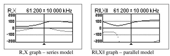
In these graphs, positive values of reactance (X) correspond to inductive load, while negative values correspond to capacitive load. Please notice the difference in the plots when the series or parallel model of impedance is selected through the *Settings* menu.
