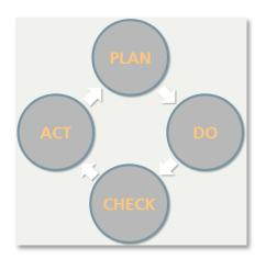
In the Check phase, the team reviews the test, analyzes the results, and identifies what has been learned. During this phase, the team measures the effectiveness of the solution and determines whether it can be improved in any way.
