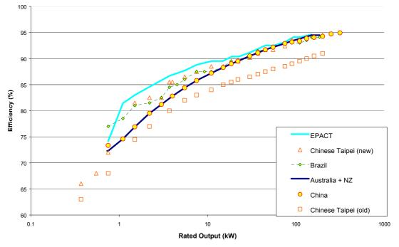
Figure 5: Comparison of Minimum Efficiency Requirements for 4 pole Motors
