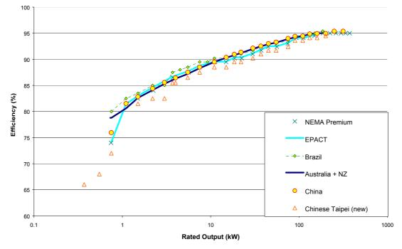
Figure 8: Comparison of High Efficiency Requirements for 2 pole Motors
