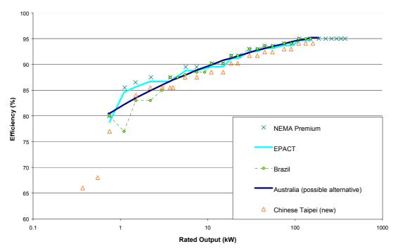
Figure 12: 6-pole high efficiency with alternative Australian values
