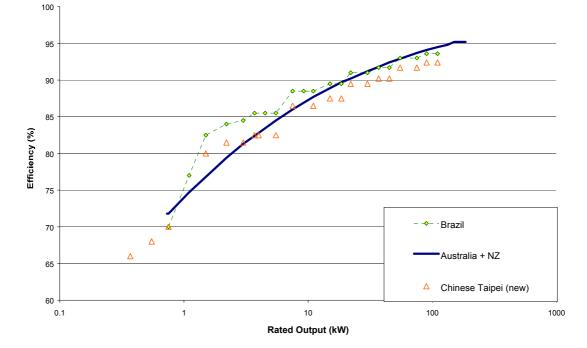
The alignment in the case of 6-pole and 8-pole motors is not so tight. However, it is possible that more stringent levels may be justified for 50 Hz 6-pole motors. Australia is considering setting a future MEPS for 6-pole motors at a level higher than the current high efficiency level. In this case, the levels are likely to be similar to those shown by the modified curve in Figure 12.
