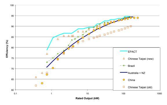
Figure 6: Comparison of Minimum Efficiency Requirements for 6 pole Motors
