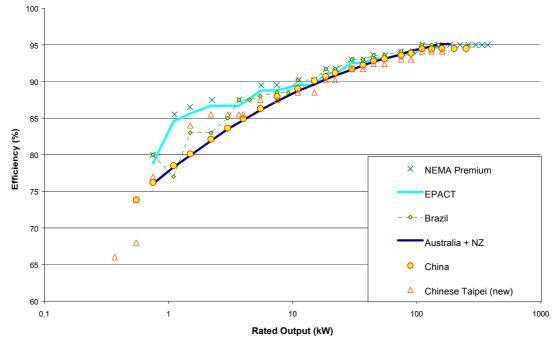
Figure 11: Comparison of High Efficiency Requirements for 8 pole Motors
