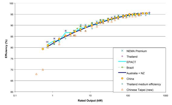
Figure 8 and Figure 9 show that for 2-pole and 4-pole motors requirements for high efficiency motors are all very similar. It is likely that these levels will become mandatory in some economies in a few years time. As well as North America, which
