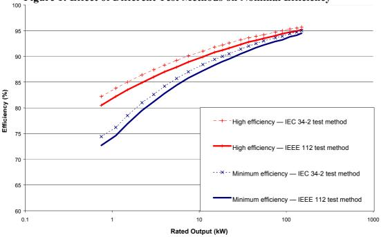
**Figure 1: Effect of Different Test Methods on Nominal Efficiency**
