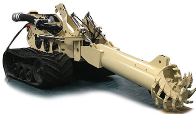
Figure 28. Submersible dredge. The cutter head for this one has as a diameter of about 1.5 feet but smaller cutter heads can be used (Eddypump.com).
