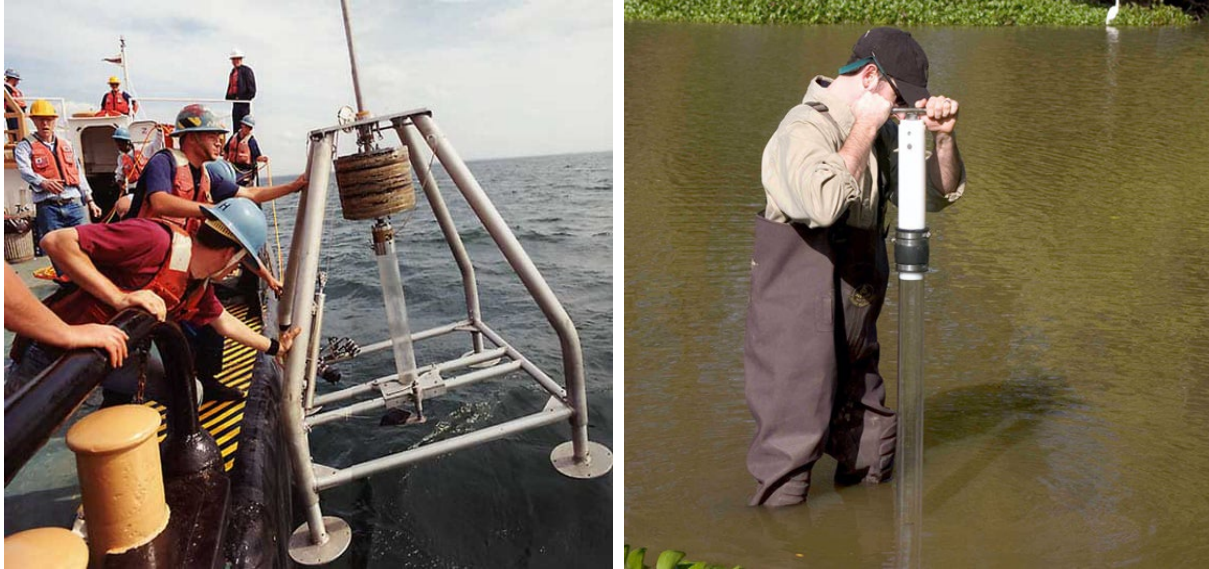
Figure 18. Left: Core samplers deployed from a vessel with a heavy frame and winch. Photograph courtesy of the Dann Blackwood, U.S. Geological Survey, Woods Hole, MA. Right: Push coring in shallow water. Photograph courtesy of WaterMark.
