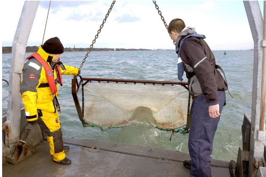
Figure 26. A bottom trawl such as the one above may be an effective SOM recovery method if the SOM is not buried very deeply. Photograph courtesy of Discover Oceanography.
