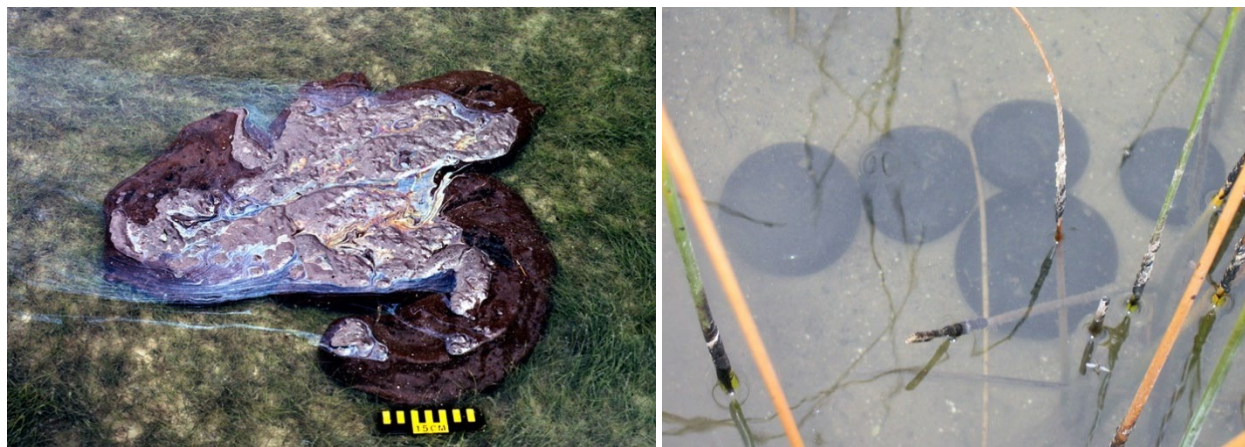
Figure 8 Left: Oily SOM is floating just below the surface from the Bouchard 65 in Tampa Bay, FL. Right: Oily SOMs in the form of rounded “tarballs” on the bottom of Lake Wabamun (Fingas et al., 2006).
