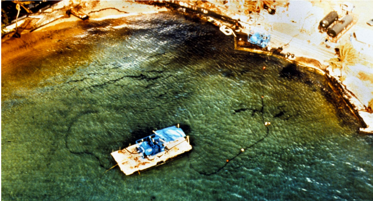
Figure 22. Barge-mounted vacuum transfer unit with diver-directed pumping during the Morris J. Berman oil spill response.
