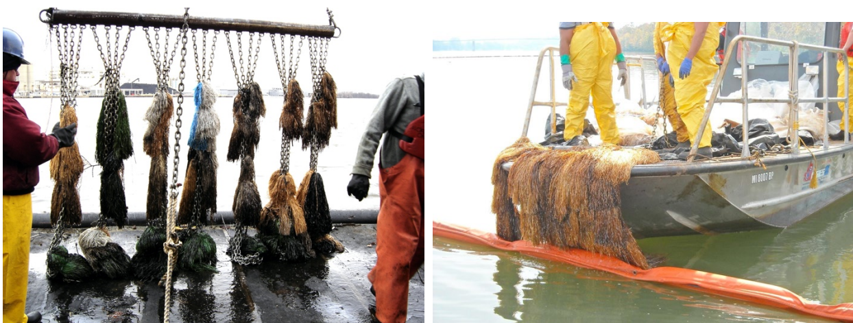
Figure 19. Left: Towed sorbent deployed using a header pipe to increase the surface areas sampled during the Athos spill in the Delaware River. Right: Towed sorbents deployed during the spill of a heavy fuel oil in the Ohio River. Photographs courtesy Mark Ploen, QualiTech.
