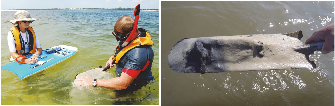
Figure 20. “Snorkel SCAT” SOM detection during the Deepwater Horizon response.
