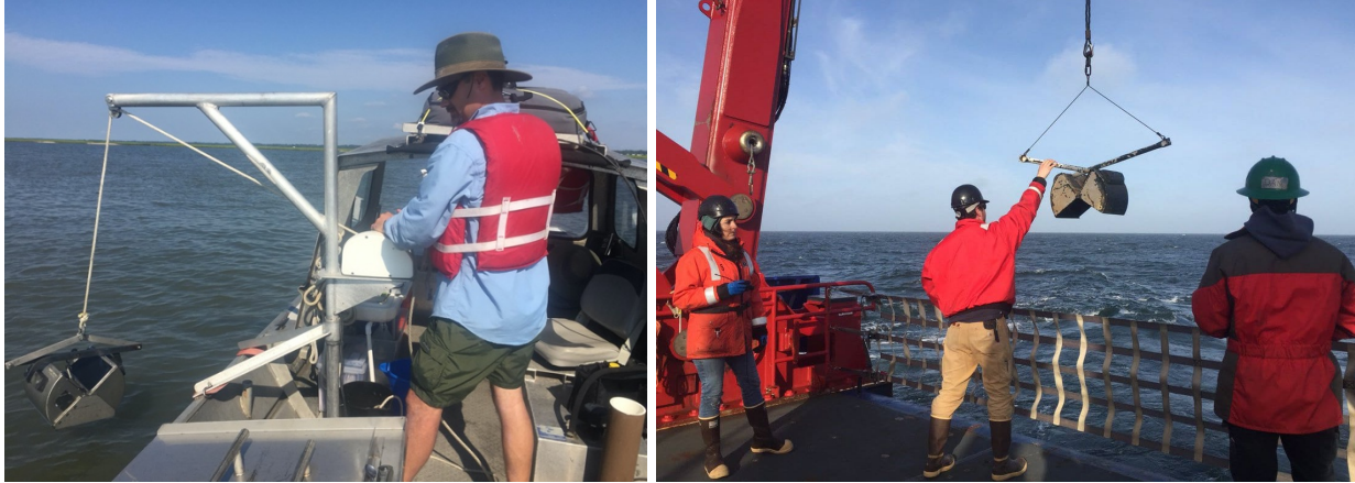
Figure 17. Left: Ponar grab sampler; Right: Van Veen grab sampler. Note that the area sampled is small.
