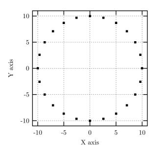
Fig. 9: Layout of the circular microphone array.
