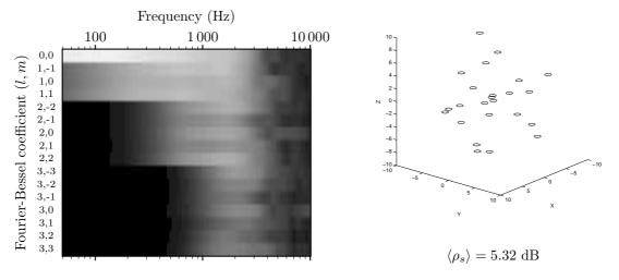
Fig. 15: Spatial signal to noise ratio for a full three dimensional microphone array.
