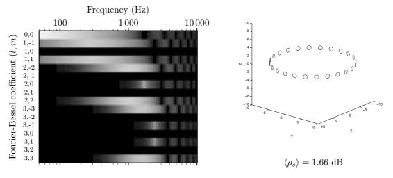
Fig. 13: Spatial signal to noise ratio for a circular microphone array.
