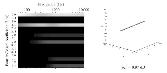
Fig. 12: Spatial signal to noise ratio for a linear microphone array.
