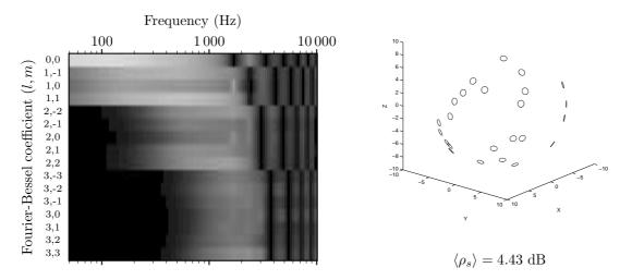
Fig. 14: Spatial signal to noise ratio for a spherical microphone array.
