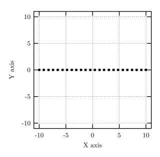
Fig. 7: Layout of the linear microphone array.
