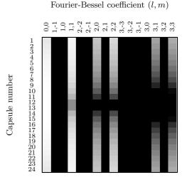
Fig. 8: Matrix B for a linear microphone array.
