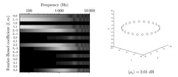
Fig. 16: Spatial signal to noise ratio for a circular microphone array with cardioid capsules.
