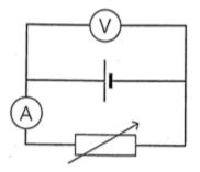
Starting with the variable resistor at its highest value (to minimize any heating effect), record the current I in the cell and the potential difference, V across its terminals for different settings of the rheostat.
