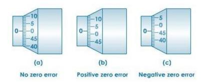
zero error = how many no. of division below or above the detum line is the zero line  $\times$  least count diameter = total reading - (±e)
