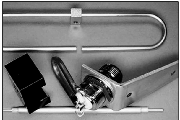
Fig. 2: Parts for the dipole; bottom: a piece of UT141-CU for the balun
