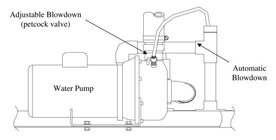
FIGURE 9-1 Water Pump / Blowdown Assembly
