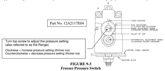
The following procedure is recommended for initially setting a freezer pressure switch that has **not** been previously adjusted (See FIGURE 9-2):
