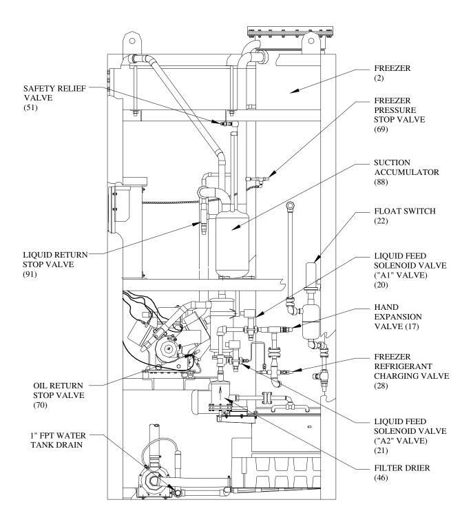
FIGURE 1-5 Assembly (Water Cooled) Right Side View
