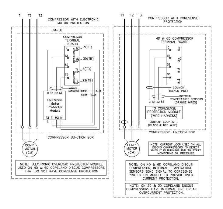
FIGURE 6-4 Compressor Schematic Detail All Voltages, 50-60 Hz.
