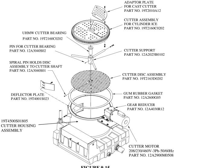
FIGURE 9-15 Cutter Parts (cylinder ice)
