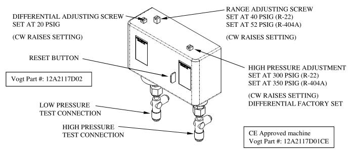
FIGURE 9-4 High-Low Pressure Switch
