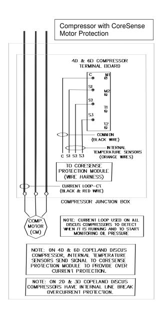
FIGURE 9-6 Compressor Protection Wiring
