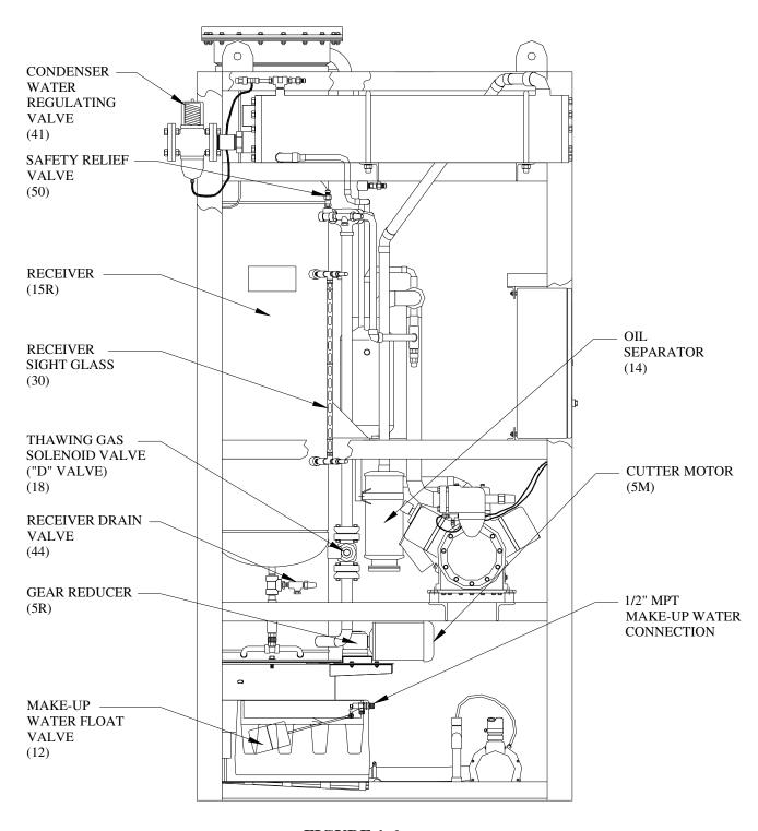
FIGURE 1-6 Assembly (Water Cooled) Left Side View
