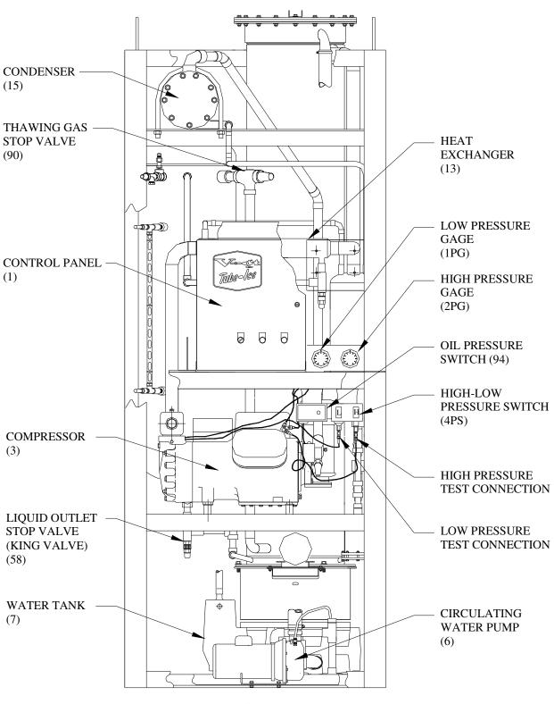
FIGURE 1-4 Assembly (Water Cooled) Front View
