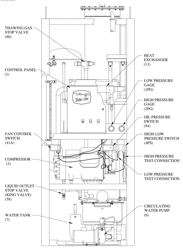
FIGURE 1-1 Assembly (Air-Cooled) Front View
