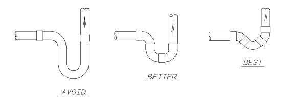
FIGURE 3-6 Minimum Traps For Discharge Lines
