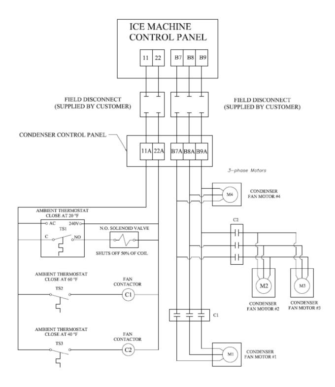
FIGURE 3-7 Wiring For BOHN BNHS04A029 with Cold Weather Valve and Four Fans, 50/50 Condenser Split
