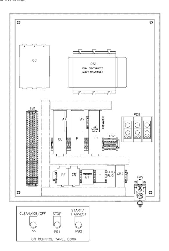
FIGURE 6-2B Control Panel Components (CE & Australian Approved)
