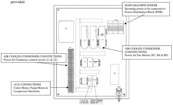
FIGURE 3-3 Control Panel Power Connections
