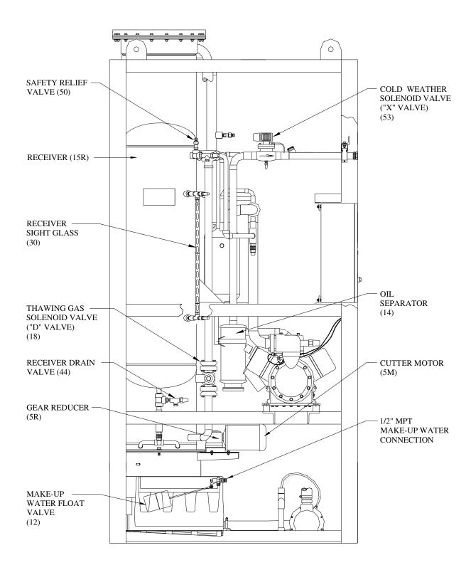
FIGURE 1-3 Assembly (Air-Cooled) Left Side View
