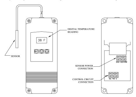
FIGURE 3-9 Electronic Thermostat
