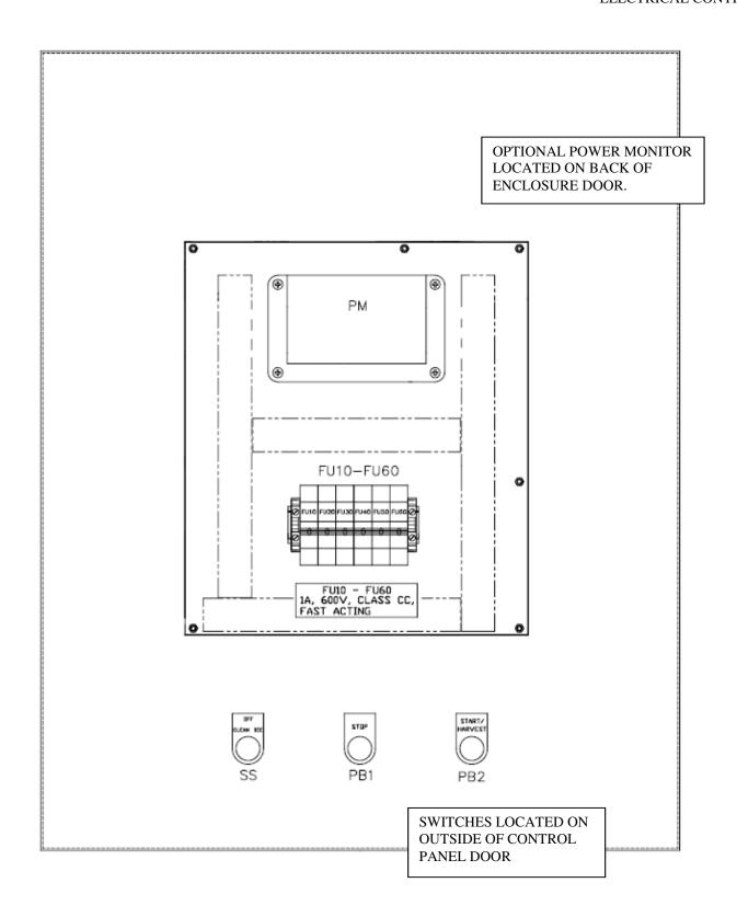
FIGURE 6-2A Control Panel Door (Standard) and Optional Power Monitor
