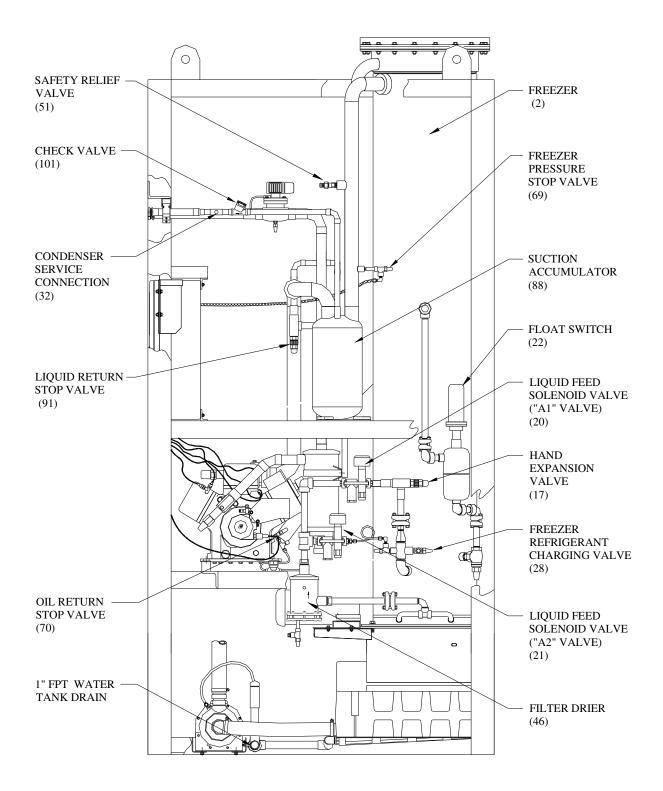
FIGURE 1-2 Assembly (Air-Cooled) Right Side View
