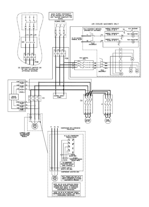
FIGURE 6-3A 3-Phase Power - Electrical Schematic All Voltages, 50-60 Hz.
