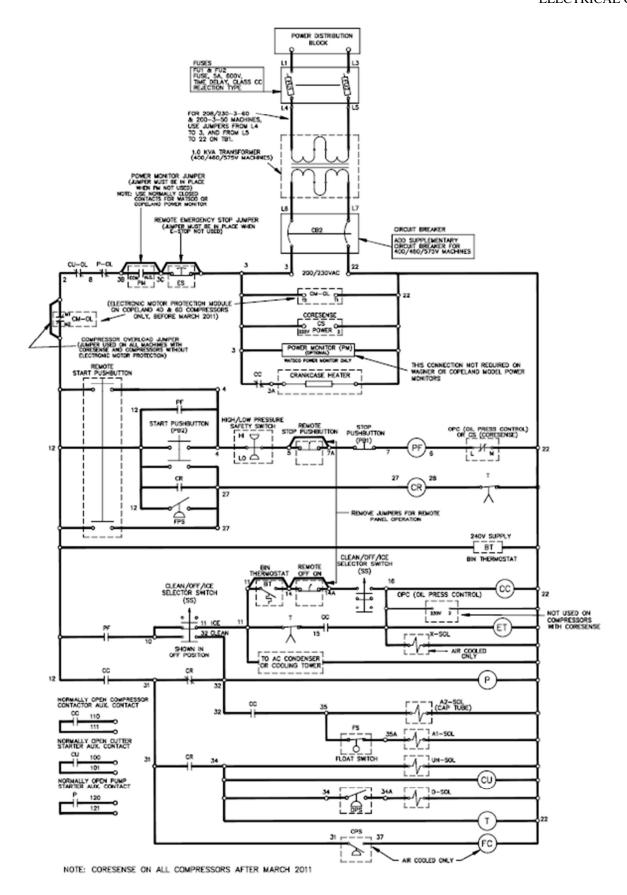
FIGURE 6-3 Control Circuit - Electrical Schematic All Voltages, 50-60 Hz.
