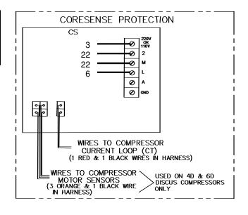
**FIGURE 9-7B**CoreSense Protection
