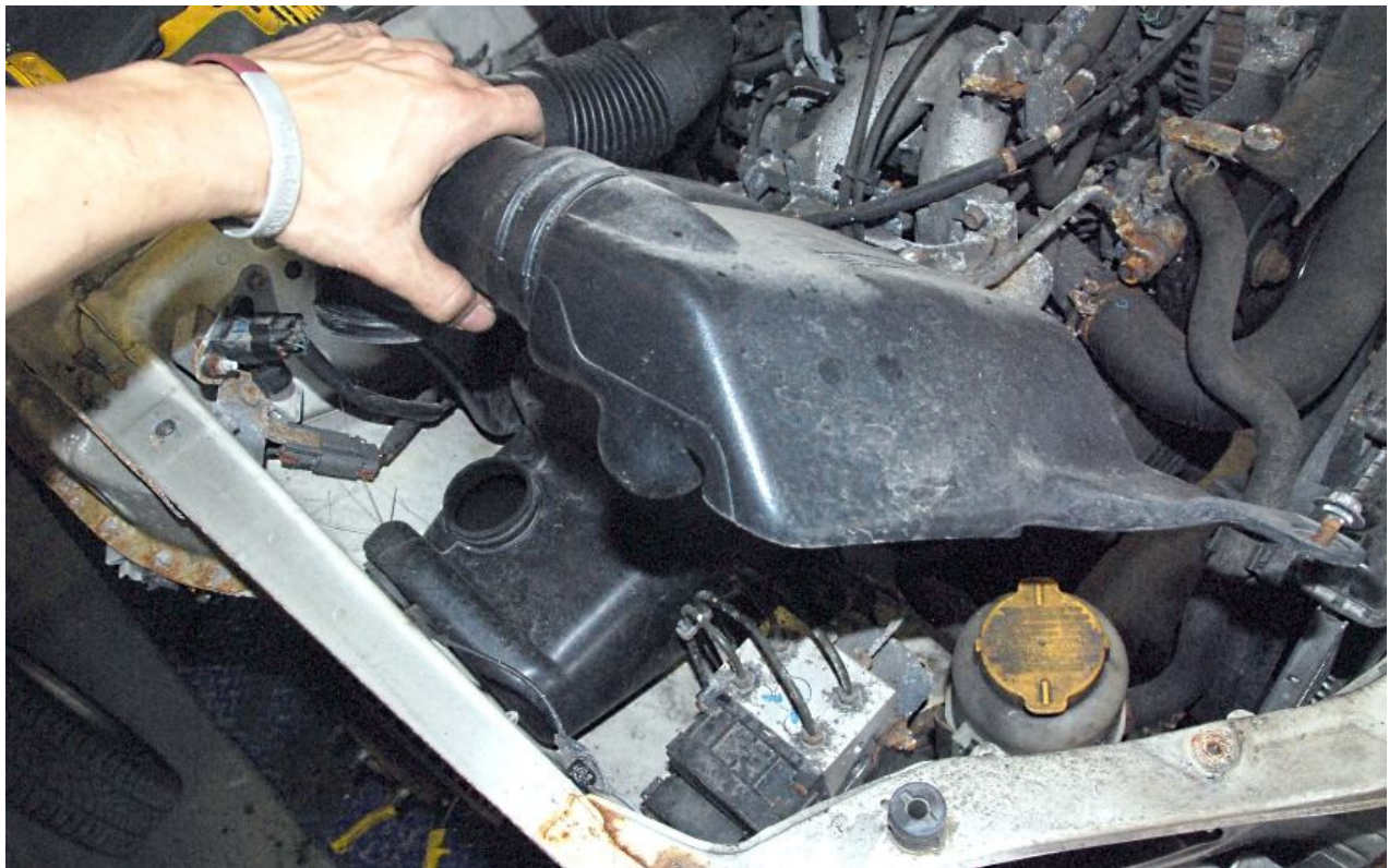
Remove the Air box and set aside for use in the build.
