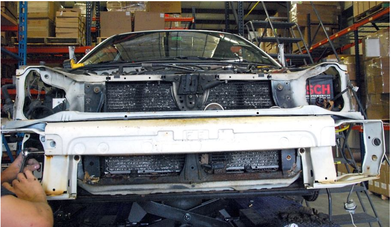
Remove front bumper cover and support.
