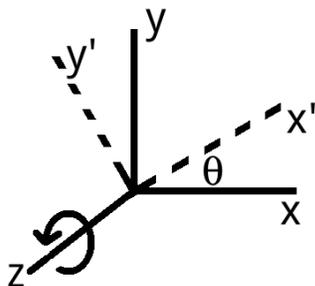
Figure 1.1: Frame rotated by an angle  $\theta$
