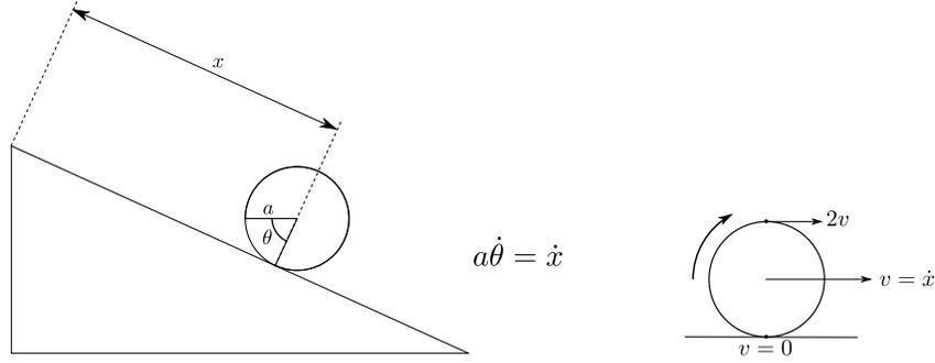
Figure 1.8: Disk rolling down an incline without slipping
