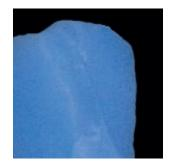
Sintered aluminum oxide
