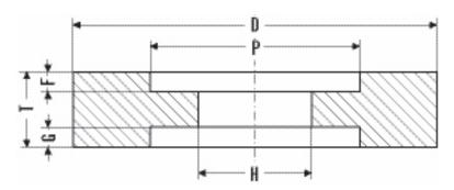
Caution: The grinding wheel may only be weakened to one half the thickness of the wheel by gouges.
