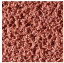
40A120 L15VPMF302W Medium-fine porosity for OD grinding
