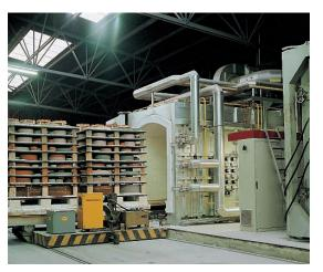
Kilns with electronic control of the temperature curve for reproducible and documented quality.
