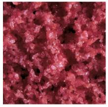
57A46 H18VPHHGG900W Highly porous structure with large pores for the highest material removal rates; mainly for hard-to-grind parts from aerospace industry
