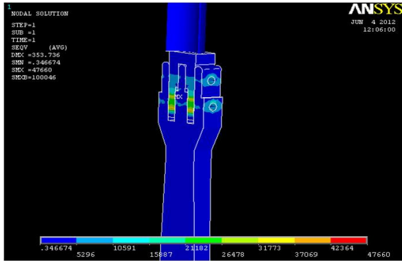
Fig.9 Von Mises stress for 3600rpm
