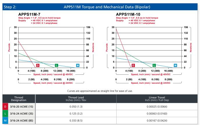
Motor step rate calculation: Motor step rate (halfstep/sec) = [Speed (in/sec)\*2] / [travel (in/fullstep)]
