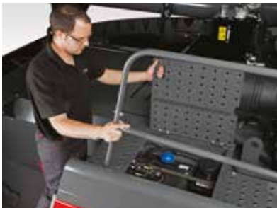
Easy refuelling - both tanks are located next to each other for easy access
