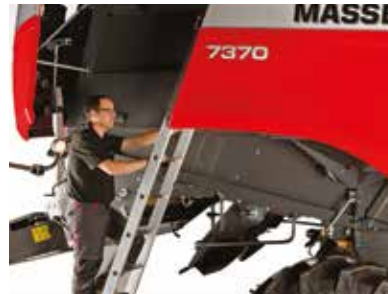
Safe engine compartment and grain tank access with removable ladder
