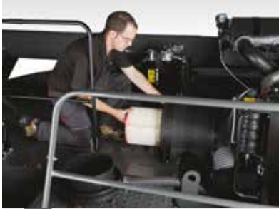
Checking and cleaning the air filter
