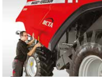
One piece panels with lights allow for quick inspection access
