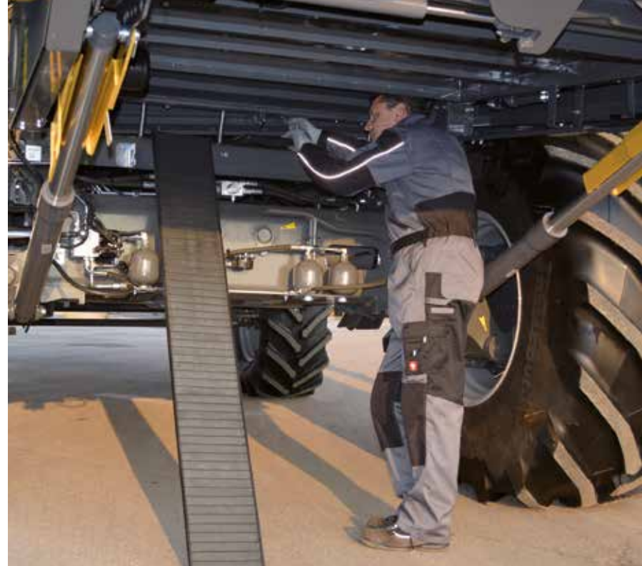
Easy access to new removable grain pan sections for quick and easy cleaning and service
