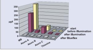
Fig. 2: Methylene blue and photoproduct reduction due to Bluflex filtration
