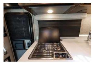
Figure 44.2 2-Burner Propane Cooktop Stove with Glass Cover Raised
