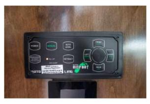
Figure 89.2 Use Leveling Control Panel to Manually or Automatically Extend and Retract Levelers
