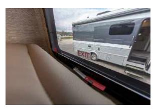
Figure 118.3 Emergency Exit Window Closed
