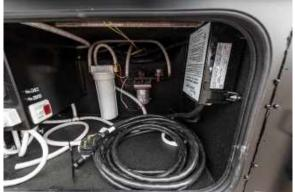
Figure 72.2 Wayfarer 30AMP Power Cord in Exterior Compartment
