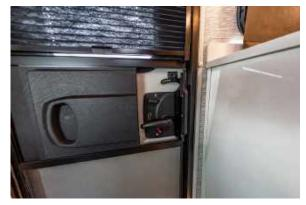
Figure 121.2 Side Entry Door Locking Mechanisms Up Close
