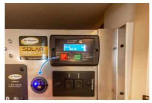
Figure 81.2 Inverter Switch Located on Central Control Panel Usually in Bedroom Area of Motorhome
