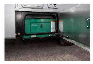
Figure 82.1 Onan 3.2kw Diesel Generator
