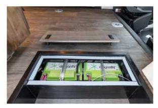
Figure 77.2 Access Panel Removed Exposing Coach Batteries \*Optional Lithium Batteries Shown
