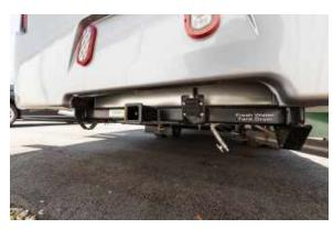
Figure 30.1 Towing Hitch and 7 Way Pin Connector
