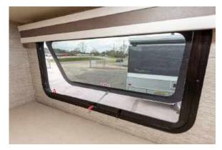
Figure 118.4 Emergency Exit Window Handle Engaged
