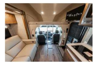
Figure 66.4 To Access Over Cabin Bunk Bed, Use Portable Ladder \*Note Bunk Bed is Rated for 500 Pounds Maximum
