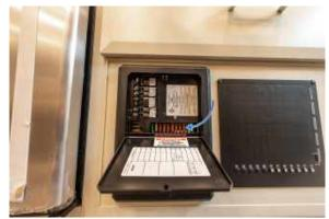
Image 64.1 Fuse That Controls the Power to the Tri-Fold Sofa Power System
