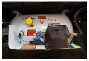
Figure 39.1 LP Propane Gas Tank
