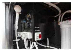
Figure 106.1 Water Pump Switch Located in Exterior Rear Compartment Drivers Side
