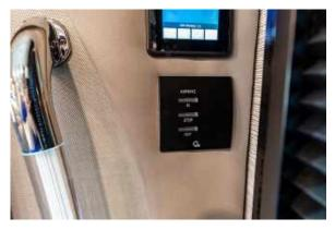
Figure 119.3 Awning Control Switch
