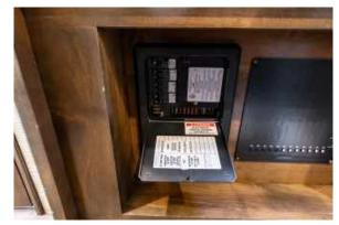
Figure 75.1 Wayfarer 120VAC Breaker and Fuses Located in Bedroom Area of Motorhome
