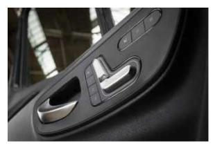
Figure 65.1 Mercedes Benz Power Seat Controls
