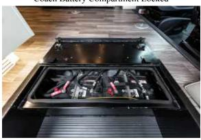
Figure 76.3 Battery Compartment Unlocked to Access Battery Distribution Center
