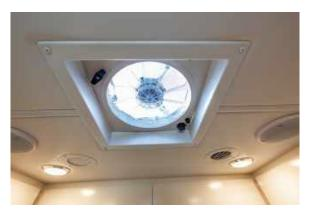
Figure 120.1 Overhead Vent Fan
