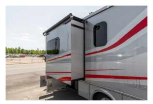
Figure 64.4 Slide-Out Room Extended
