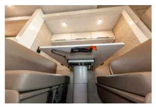
Figure 61.3 Pull On Lever Under Table To Release
