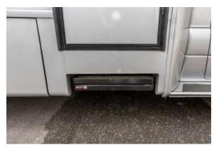
Figure 98.1 Side Entry Exterior Power Steps in Retracted Position
