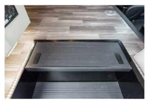
Figure 77.1 Coach Battery Located Inside Entry Step Well
