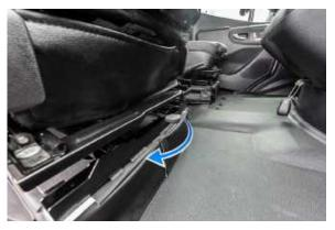
Figure 65.2 To Rotate Seats, Push Release Lever Towards Door and Start Rotating the Seat Inwards
