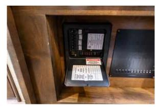
(Figure 84.1) Circuit Breaker Box Located in Bedroom Area of Motorhome
