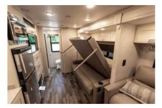
Figure 63.4 Power Tri-Fold Sofa Partially Opened with Legs in Down Position.
