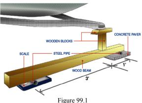
To Measure Tongue Weight, Utilize Components Shown. Multiply Weight on Scale By Number of Feet Scale is From Center of Tongue. In Image Above, Scale Is 3 Feet From Center of Tongue. Multiply Weight On Scale By 3.
