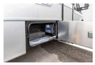
Figure 96.2 Exterior Compartment Which Also Houses Components Necessary to the Motorhomes Function. NOTE: Use Caution When Storing Items in These Compartments to Avoid Damaging Motorhome Components
