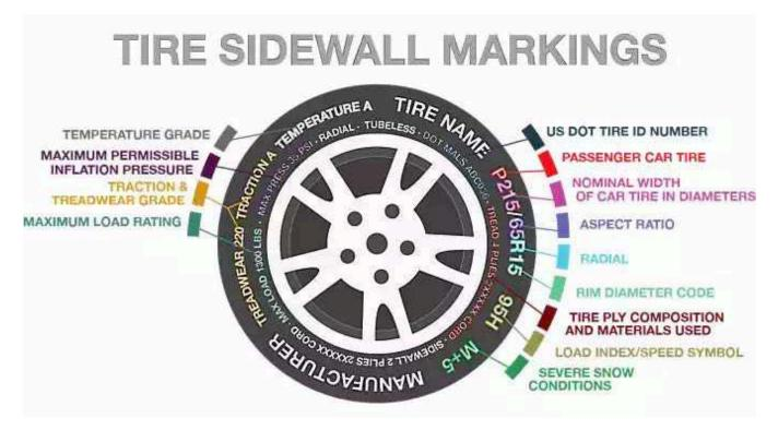
The image above provides an example summary of the sidewall markings on passenger vehicle tires.
