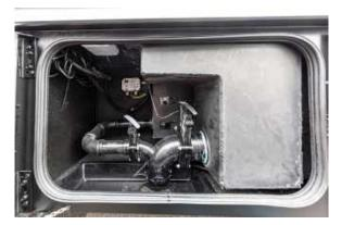
Figure 114.1 Sanitation Coupling with Gray and Black Water Tank Gate Valves NOTE: This Unit Can Be Found In An Exterior Storage Compartment Located On the Drivers Side of the Motorhome
