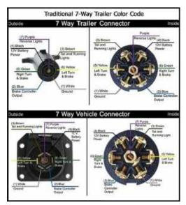
Figure 85.2 7 Pin Connector Wiring Diagram
