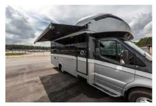
Figure 119.2 Power Awning In Extended Position
