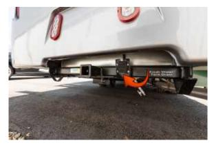
Figure 85.1 7 Pin Connector on Tow Hitch
