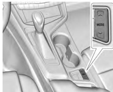
Driver Mode Control Switch
