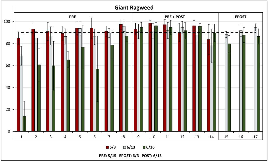
**Figure 1**: Giant ragweed efficacy ratings for trial #19-ROK-CN02. Bars indicate the average % control ± the standard deviation of four replications following herbicide applications. Numbers on the x-axis correspond to the herbicide treatment list for the respective trial number. The dashed line indicates 90% control.
