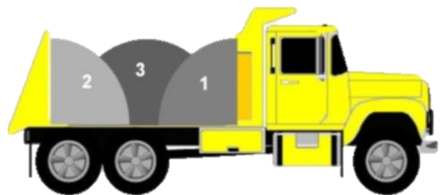
Figure 43 – Correct Truck Loading Scenarios
