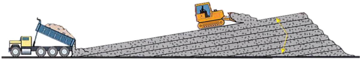
Figure 23 - Building a Stockpile in Layers
