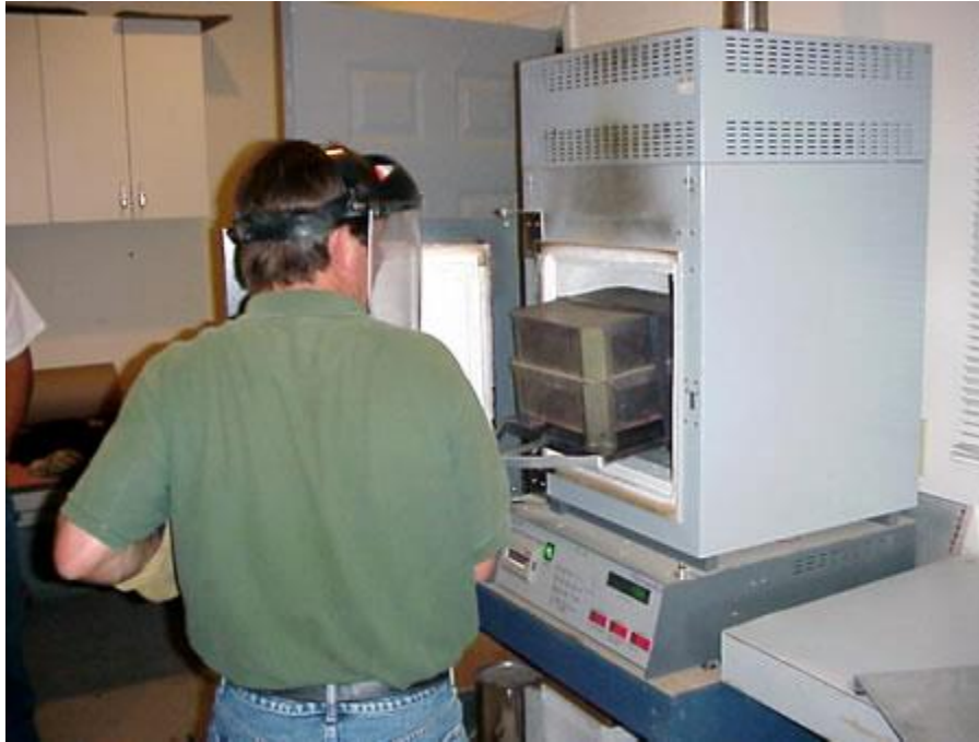
Figure 68 - Determining Asphalt Content using NCAT Ignition Oven
