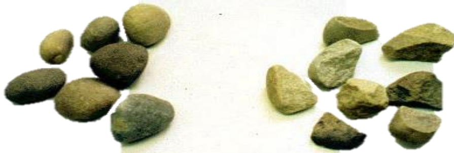
Figure 34 - Difference between river gravel before and after crushing
