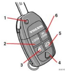
*Buttons in remote control:* 1 -Fold key in/out, 2 - Lock, 3 - Approach lighting, 4 - "Panic" function, 5 - Unlock tailgate, 6 - Unlock
