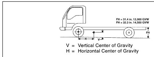
The center of gravity of the completed vehicle with a full load should not exceed 54 inches above ground level for the 12,000 lb. GVWR, 58 inches above ground level for the 14,500 lb. GVWR, and must be located horizontally between the centerlines of the front and rear axles.
