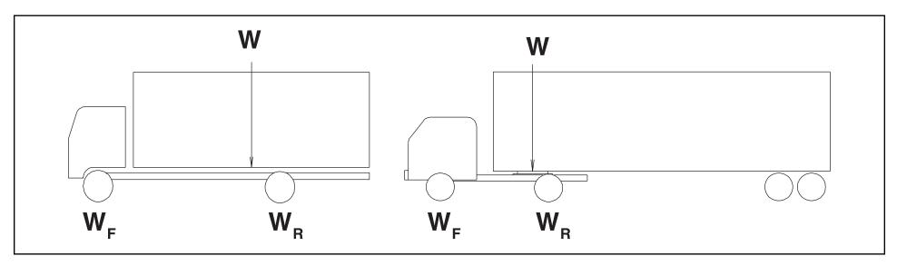
The weight at the center of the body and the load when applied is the same as the single point load of the kingpin on the fifth wheel.
