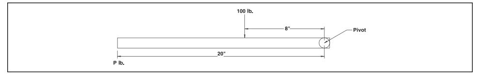
To find the value of "P", the leverages must be equal for balance.
