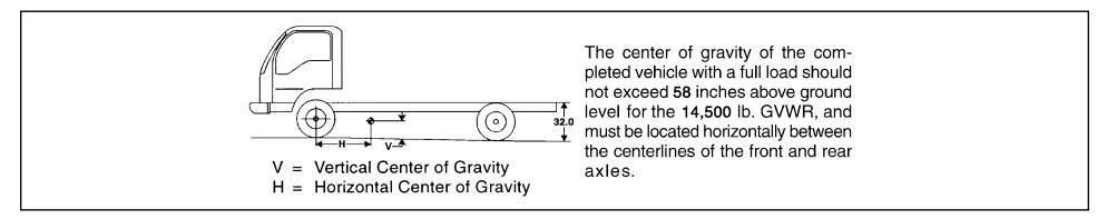
**NOTE:** The maximum dimensions for a body installed on the NQR/W5500 are 96 inches wide (outside) by 90 inches high (inside). Any larger body applications must be approved by GM/Isuzu Application Engineering. In the West Coast call 1-562-229-5314 and in the East Coast call 1-404-257-3013.
