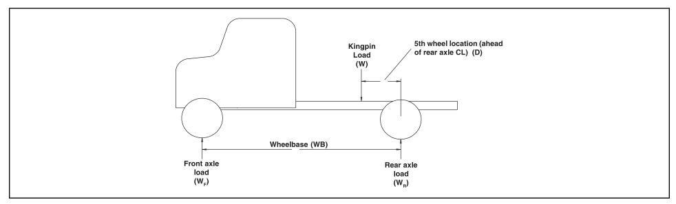
Front Axle Load: = Kingpin Load x 5th Wheel Location Wheelbase
