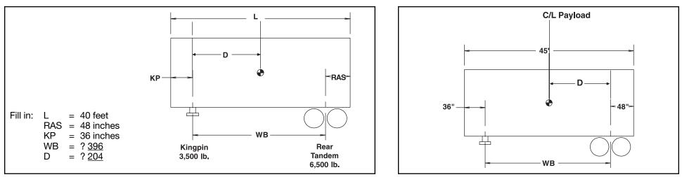
In the following example, a 50,000-pound payload at water-level loading. Calculate the payload (PL) weight transfer to kingpin and the rear axle.
