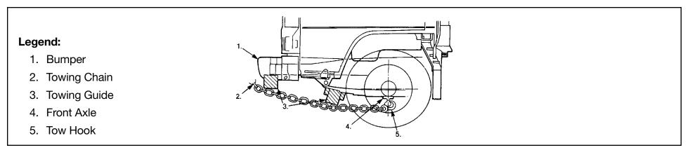
To prepare a disabled vehicle for front end towing with all wheels on the ground, the following steps are necessary:
