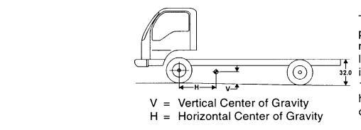
The center of gravity of the completed vehicle with a full load should not exceed 54 inches above ground level for the 12,000 lb. GVWR, 58 inches above ground level for the 14,500 GVWR, and must be located horizontally between the centerlines of the front and rear axles.
