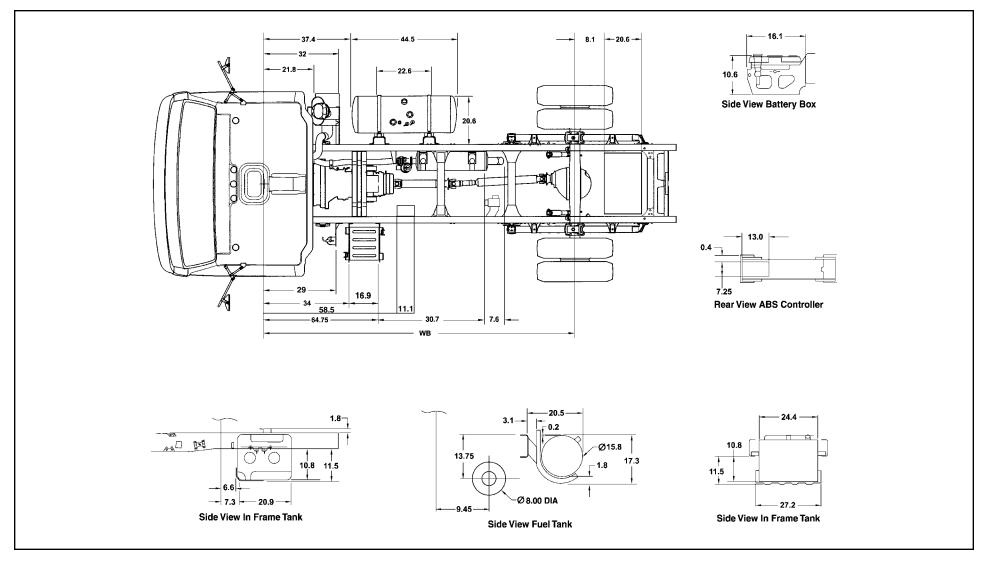
**NOTE:** Frame-mounted fuel tank available on 109", 132.5", 150" and 176" WB as an option replacing the In-Frame Tank. \* Allow 3" additional for battery box opening clearance.
