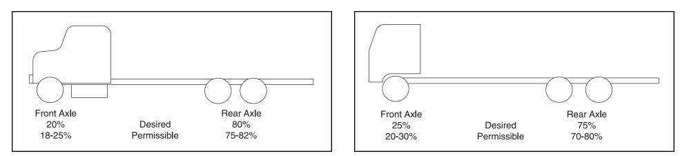
Calculating tractor/trailer weight distribution can be thought of in the same terms as calculating full trucks.
