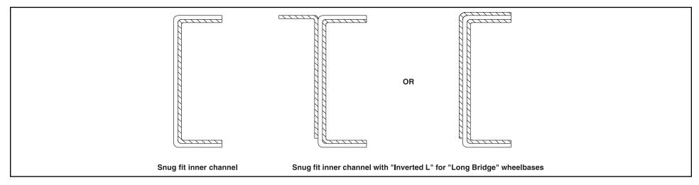
7. The reinforcements must be fastened securely to <u>only</u> the web of the original chassis frame rail. The reinforcement must be held rigidly in place using either HUC bolts, GRADE 8 bolts and hardened steel washers at <u>both</u> the bolt head and nut, or GRADE 8 flanged bolts and hardened steel washers at the nut. Below are some suggested bolt patterns. It should be noted that these bolt patterns must <u>not</u> align the bolts vertically, i.e.: the bolt pattern must be staggered.
