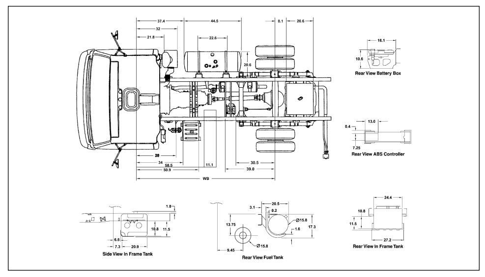
**NOTE:** Frame-mounted fuel tank available on 109", 132.5", 150" and 176" WB as an option. Allow 3" additional for battery box opening clearance.
