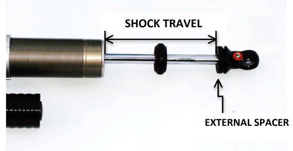
SOME SHOCKS USE EXTERNAL SPACERS BELOW THE BUMP STOP TO LIMIT TRAVEL. DO NOT INCLUDE THE SPACER LENGTH AS PART OF THE TRAVEL.
