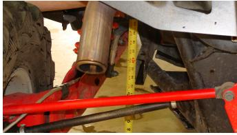
WARNING: Do not add excessive amounts of preload into the coil spring. Doing so may result in coil-bind, which could lead to spring failure and potential injury or death. To check coil-bind, put several zip-ties around individual coils. If they break or show contact, there is excessive preload. If you are at maximum preload and need more ride height, contact FOX for a stiffer spring.
