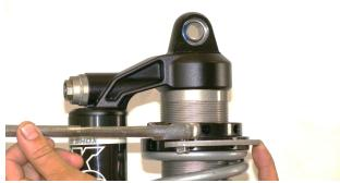
P/N 398-00-393 Tooling: Spanner, Preload Wrench
