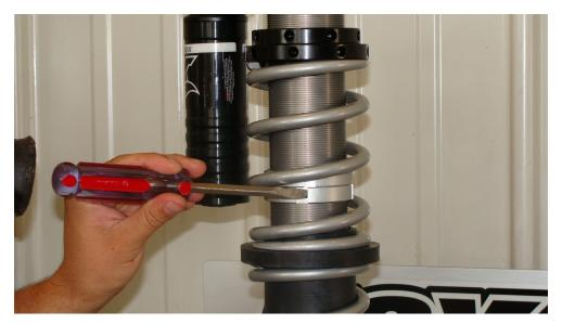
**STEP 6** Adjust the crossover ring (as shown previous page) so that its distance from the spring coupler is equal to the crossover ring placement value calculated in Step 5. Lock the crossover rings together once complete with a flat-bladed screwdriver and hammer.
