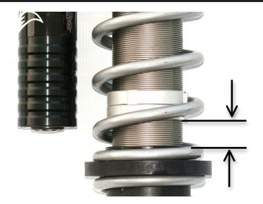
Crossover ring placement value should match the distance from the top of the spring coupler to the bottom of the crossover ring. Example .912 inches
