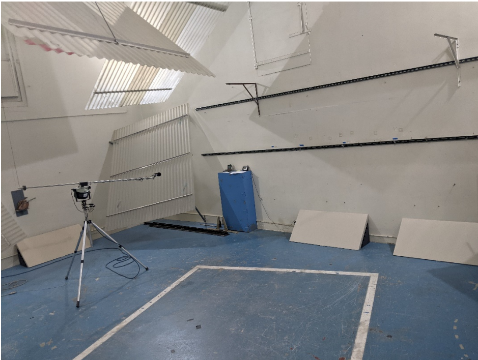
Figure 2 – Specimen configuration at east (left) and south (right) chamber walls
