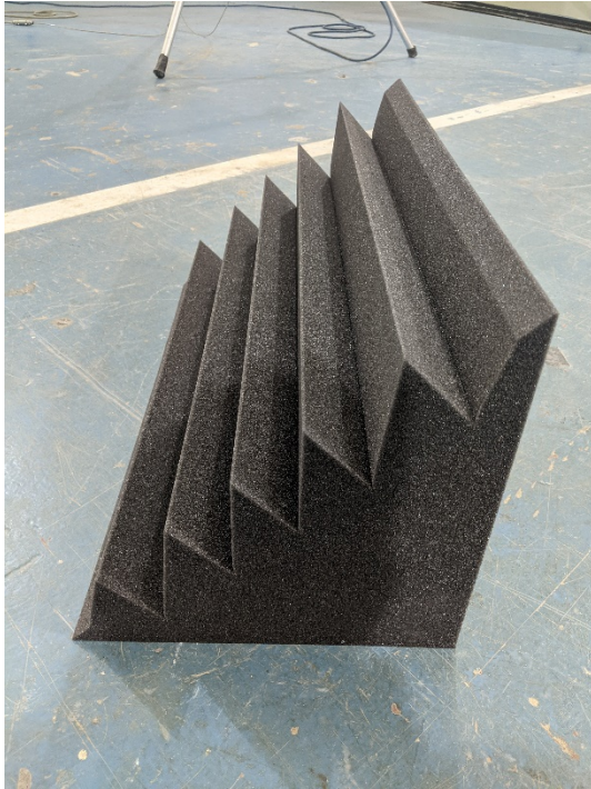
Figure 3 – Individual foam piece, sawtooth profile along diagonal
