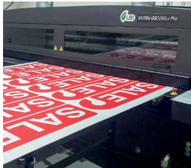
The EFI VUTEk GS3250Lx Pro prints 60 1.20 m x 2.40 m boards an hour.
