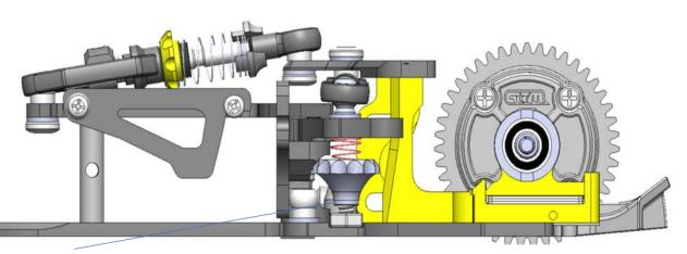
Adjust the side spring cup, to make the spring just barely touch the top plate.
